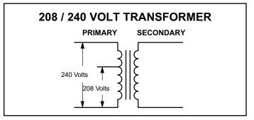
Figure 13. Converting Unit from 240VAC to 208VAC
