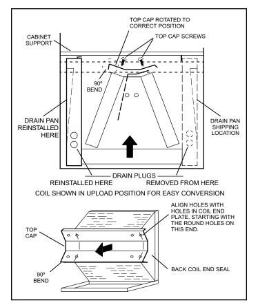
Figure 4. Field Modification for Left-Hand Discharge
