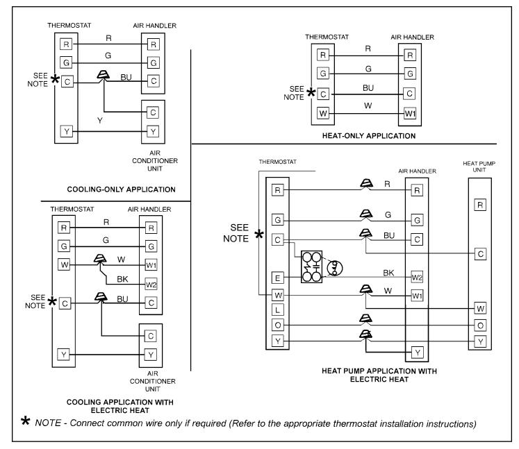
Figure 15. Low Voltage Connections (Constant Torque Motor)
