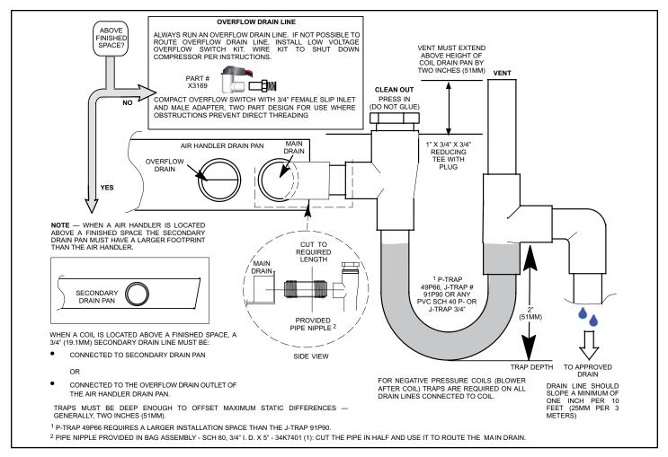
Figure 6. Typical Main and Overflow Drain
