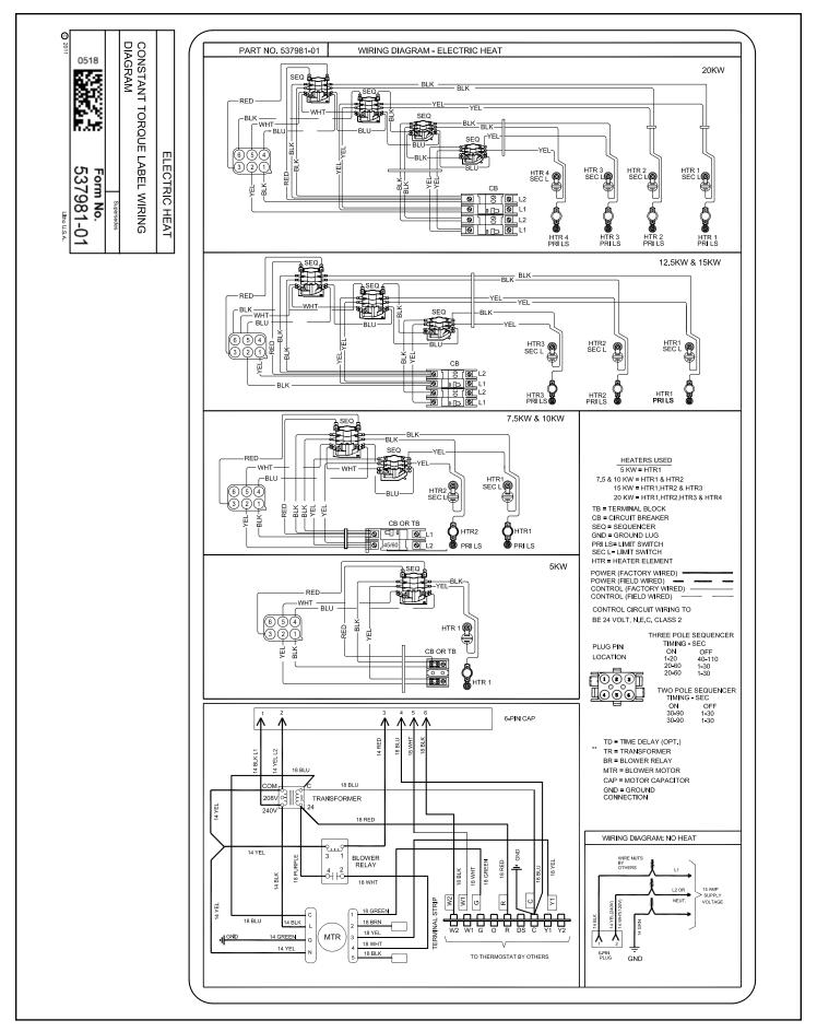
Figure 14. Typical Wiring Diagram MAHM\*ETA Air Handler with Electric Heat – (Constant Torque Motor)
