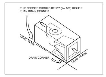
Figure 7. Sloping the Unit for Proper Drainage
