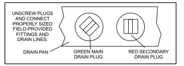
Figure 8. Drain Line Connections
