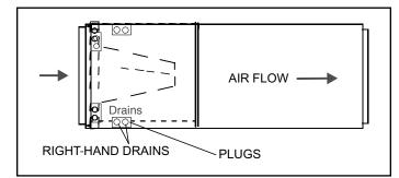
Figure 2. Right-Hand Discharge Configuration
