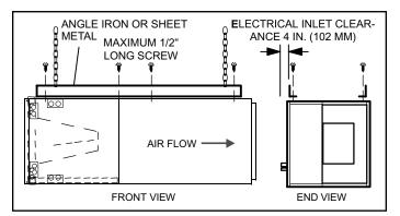
Figure 3. Suspending Horizontal Unit
