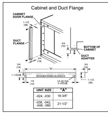
**Figure 9. Cabinet and Duct Flange**
